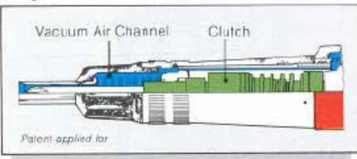
Provides greater visibility at the screwhead as bulky external vacuum fittings are not required. The integral vacuum totally bypasses the clutch, thus preventing the ingress of debris into the mechanism. This unique Desoultre feature helps to sustain clutch accuracy and prolong clutch life.
