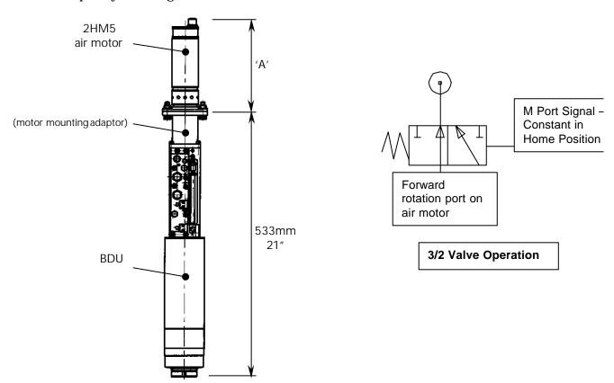
A 3/2 Valve (supplied) is required with an A1 block in order to turn the air motor off at the home position. Similarly external valves(not supplied) will be required with the A6 block.
