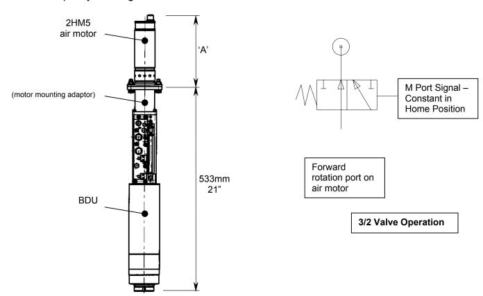
A 3/2 Valve (supplied) is required with an A1 block in order to turn the air motor off at the home position. Similarly external valves (not supplied) will be required with the A6 block.
