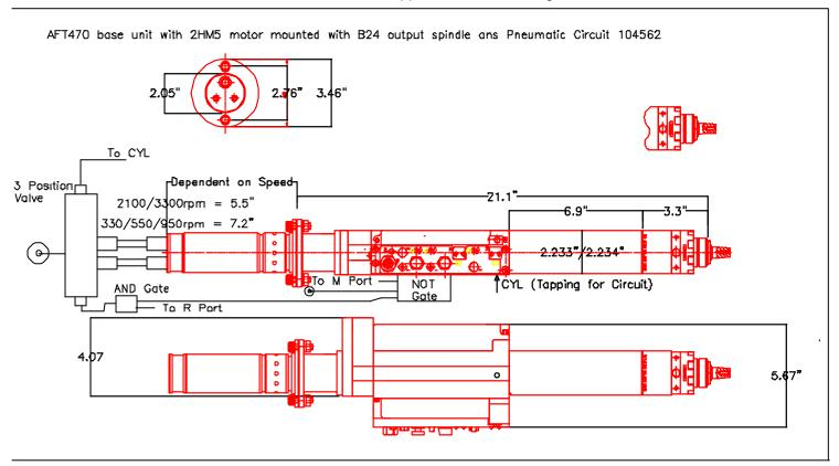
2HM5 Air Motor used in direct drive – Refer to Air Motor Catalogue LT1317 Page 9 for details on the 2HM5 Only 330rpn to 3300rpm tools to be used.
