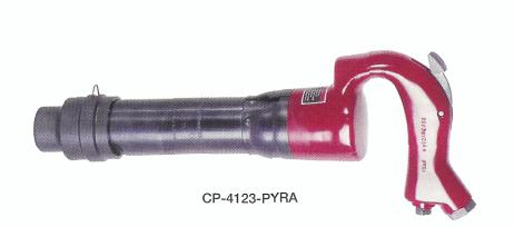
All Models: pistol grip handle with self-closing outside trigger, 3/8" (NPTF) air inlet thread; air consumption at 90 psi, 23 - 27 cfm.
