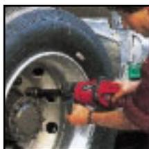
A 6" extension anvil is available for the CP6110. 1" square drive with 6" extension, friction ring retainer – part no. C144686.
