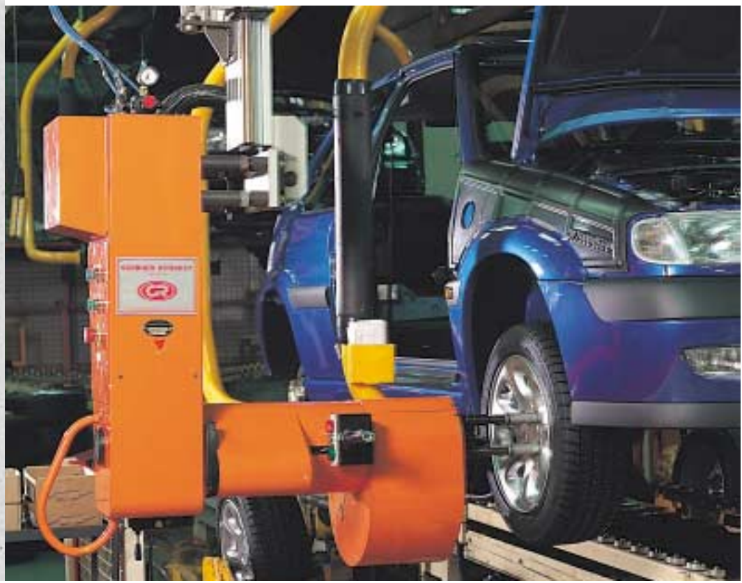
"Tightening wheel" assembly machine with 3 or 4 spindles changing (France)
