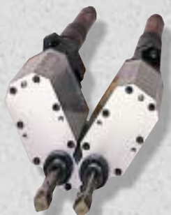
OFFSET GEAR TO REDUCE THE DISTANCE OF THE SOCKETS
