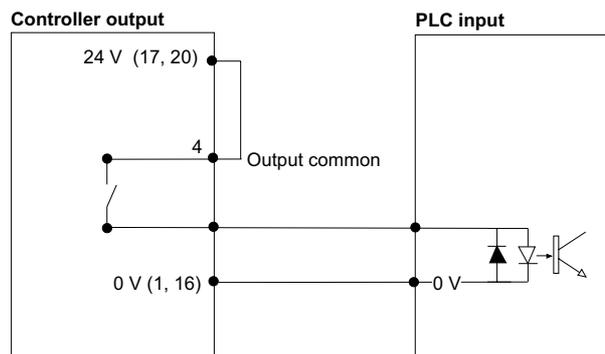
All outputs are active at 1 and relayed in the controller with a common point (4) for all outputs.
