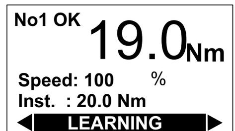
The "CALIBRATION" screen allows you to readjust the calibration to the set point of a specific tightening when the automatic calibration has not been deemed sufficient.
