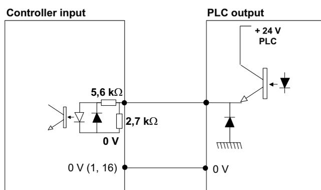
The inputs are type II as per standard CEI 1131-2 (24V/13mA per input)
