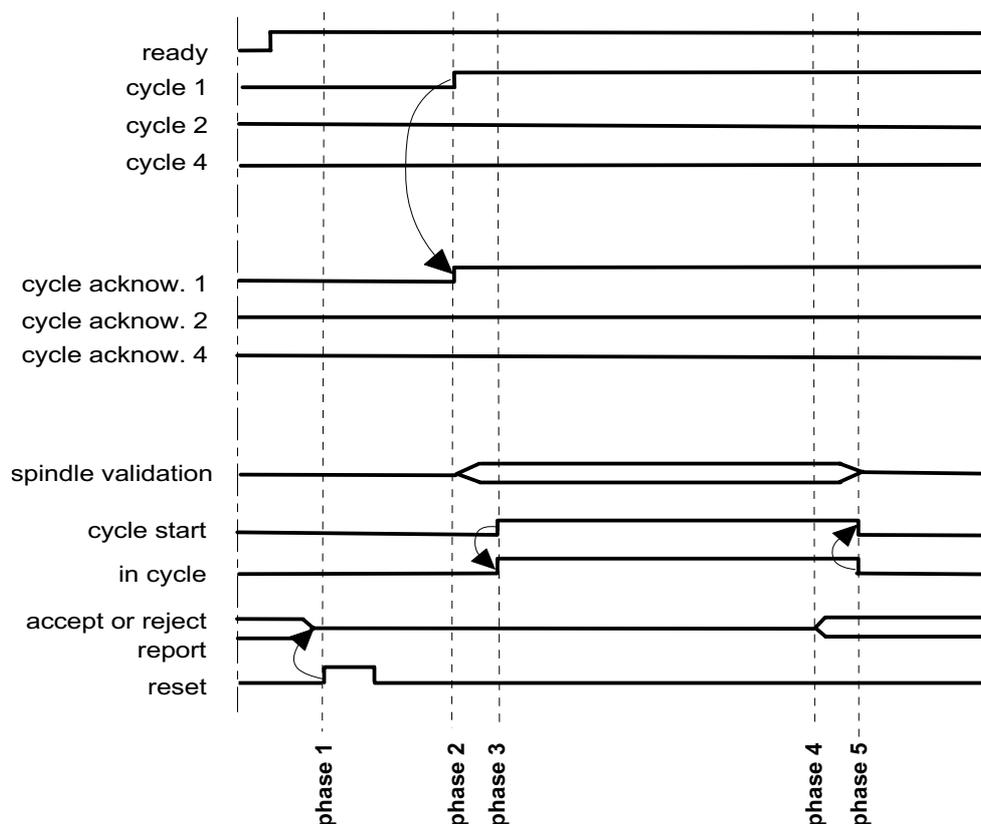
phase 1 : the controller receives cycle n°1 --> cycle acknowledgement n°1 is validated (if the cycle is programmed)
