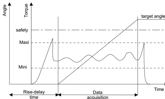
**Spindle stop** **IF** angle  $\geq$  target angle **OR** torque  $>$  safety torque
