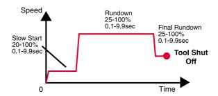
Parameters Tool start mode, external forward, reverse or stop signal functions, slow start time and speed,
