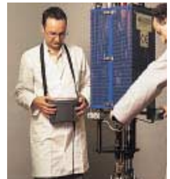
Checking the torque on multi-spindle machine
