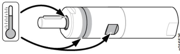
The following hotspots on the motor (as seen in the figure above) can reach high temperatures during operation:
