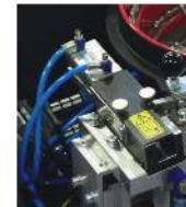
Escapement sensors Control/Secure escapement mechanism
