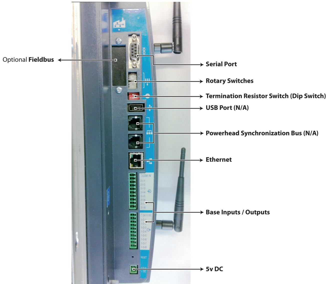
**NOTE:** The Power-head synchronization bus and USB port are not in use.
