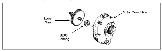
• Press the upper gear bearing (525424) and lower gear bearing (BB66) into the gear case.
