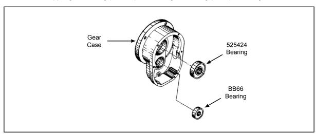
Position the gasket on the motor case plate and assemble the gear case.
